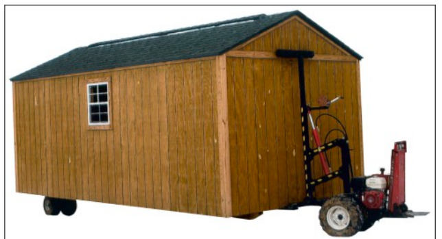
Mule: Available in most areas, used for tight areas and easier maneuvering
